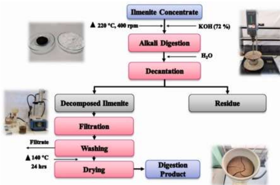
Figure 2. Flow diagram of alkali digestion process
