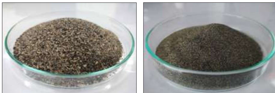
Figure 1. (a) Raw heavy mineral sand and (b) ground heavy mineral sand
